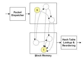
Fig. 8. Distribute graph vertices into multiple memory blocks to improve the lookup throughput. s is the starting vertex and t is the terminating vertex
