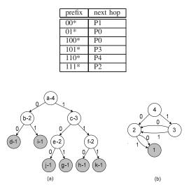
Fig. 4. Label the leaf-pushing trie with shape ids and build the shape graph
