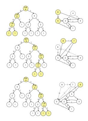
Fig. 7. Illustration of the shape graph updates as the new prefixes "001\*", "1100\*", and "1111\*" are inserted sequentially. Left side is the updated leafpushing binary trie and the right side is the updated shape graph. The dark nodes (vertices) indicate the newly inserted or updated nodes (vertices). The dashed vertices and edges in the shape graph indicate the unused vertices and edges after the update
