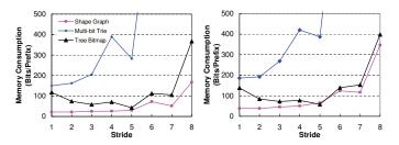
Fig. 10. Overall memory consumption comparison on two prefix tables. The left side is for AS1221 and the right side is for Maewest
