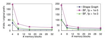
Fig. 12. Memory consumption for different number of memory blocks. The left side is for the AS1221 table and the right side is for the Maewest table.
