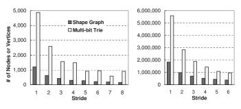
Fig. 13. The number of shape graph vertices vs. the number of multi-bit trie nodes for IPv6 forwarding tables. The left side is for the IPv6 BGP table and the right side is for the synthesized IPv6 table
